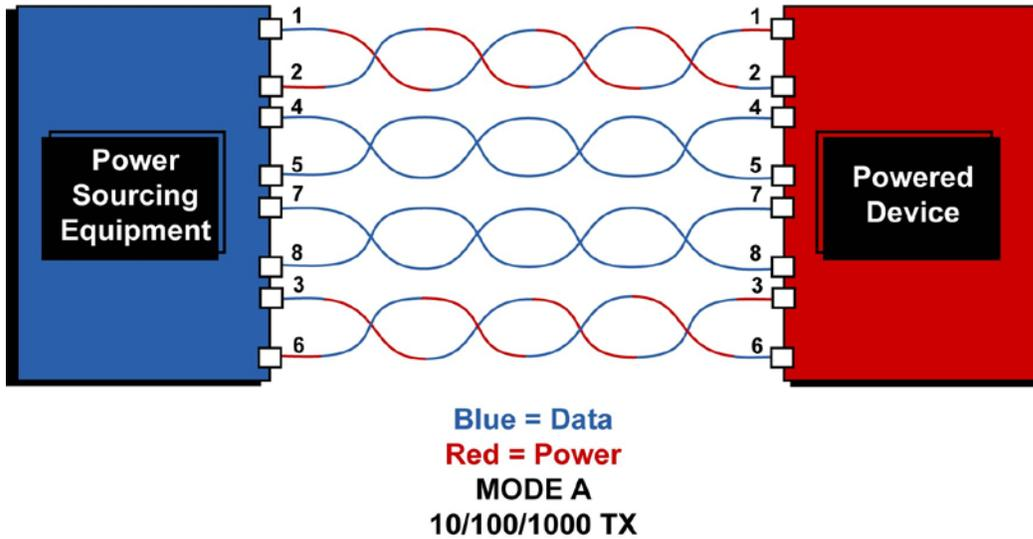
In the case of 10/100BaseT Mode A, spare pairs 4/5 and 7/8 are unused See Diagram 3.
