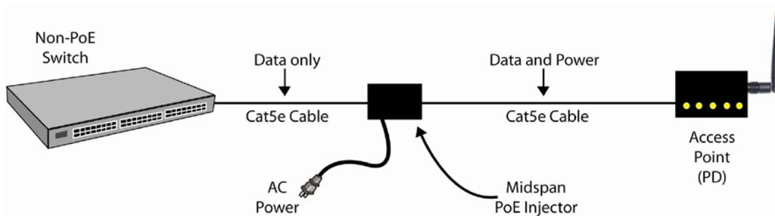
These devices can be fully compliant with 802.3af or be “Passive” and only offer power limiting. Passive MidSpans or Injectors offer lower cost as well as higher power capability and the ability to power non 802.3af compliant network appliances. In the wireless industry, to save cost or draw more power, it is common to use remote client devices that only work with passive PoE injectors.
