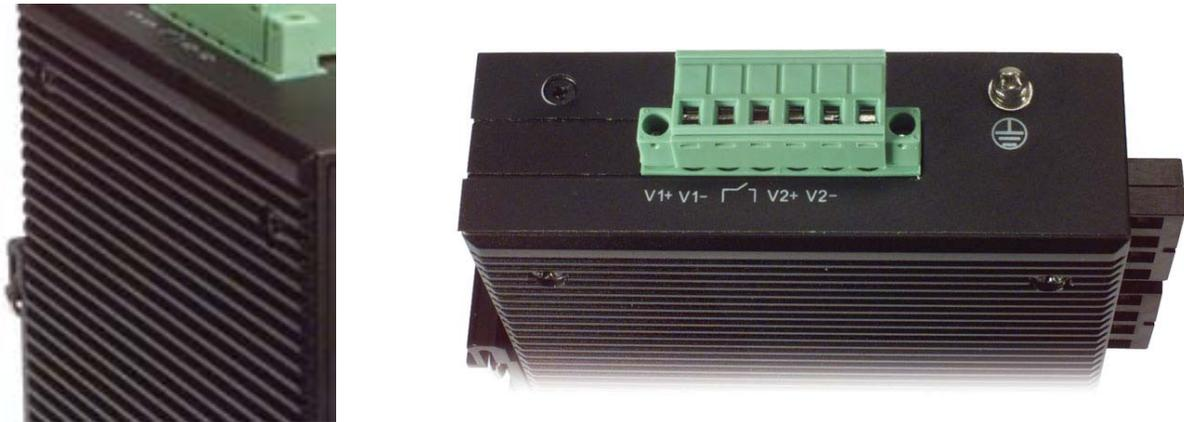
The image on the left details the case of an Industrial Ethernet Switch that acts as the heat sink for the unit. The image on the right shows dual power inputs as well as a dry contact for connecting alarm devices for visual or audio warning in the event of a power supply failure.
