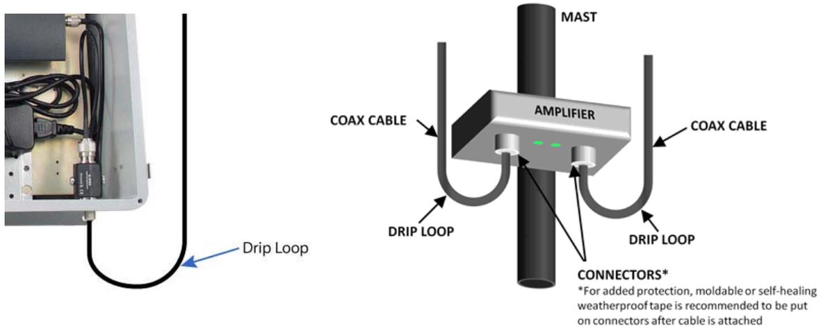
If you are using a wireless amplifier or radio it is best to position it as close to the antenna as possible (without putting too much stress on the connecting cables). Make sure the amplifier connectors are face down and leave enough room for drip loops.
