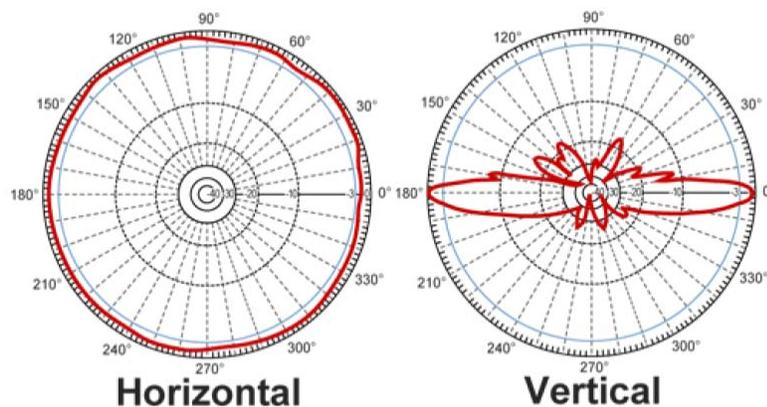
Typical Omni directional antenna radiation pattern (HG2415U-PRO)
