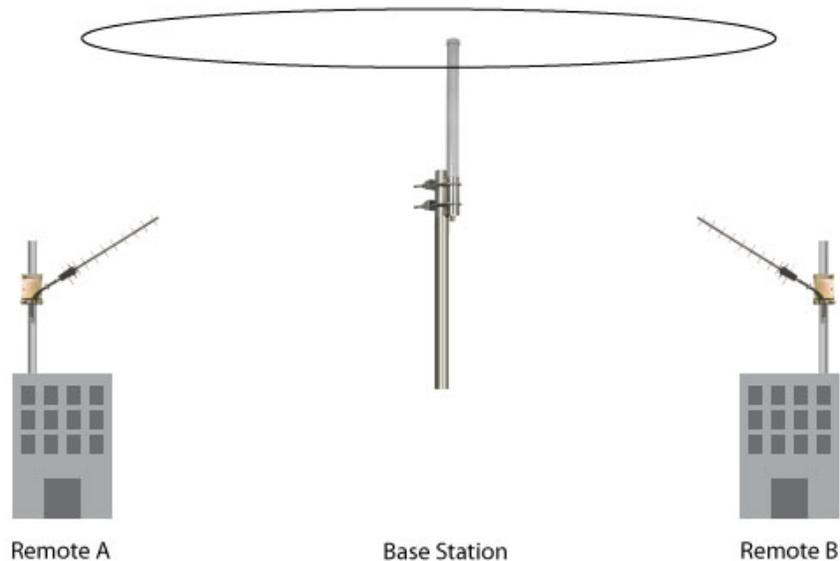
In this example both remote sites A and B have directional Wi-Fi connectivity to the base station fitted with an Omni directional antenna. This is an example of a point to multi-point set up.
