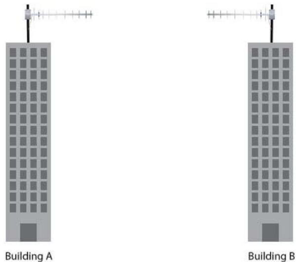
In the example above building A and building B are set up for a directional, point to point network using Yagi antennas
